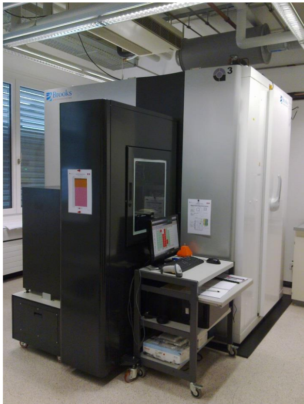
Automated storage system for tubes and plates Capacity > 200'000 compounds
